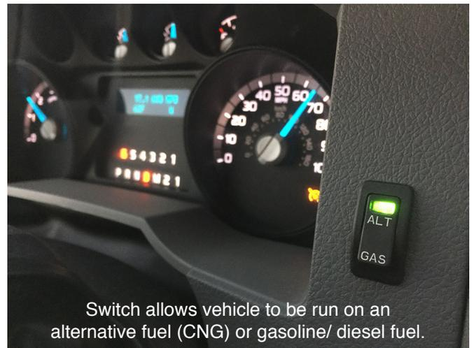
Switch allows vehicle to be run on an alternative fuel (CNG) or gasoline/ diesel fuel.
